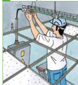
6 Connecting power to the line
