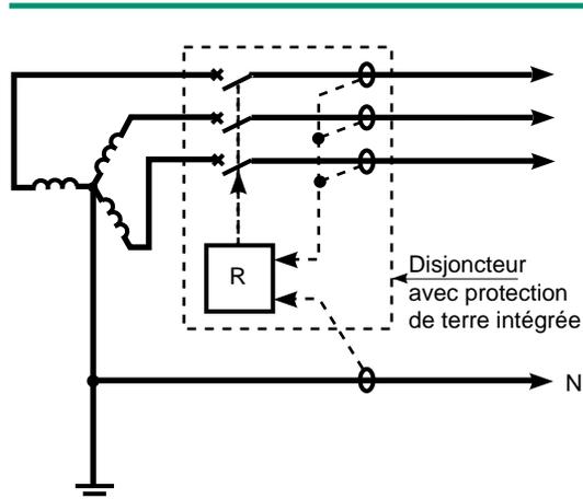
**Fig. 14** : residual sensing.
