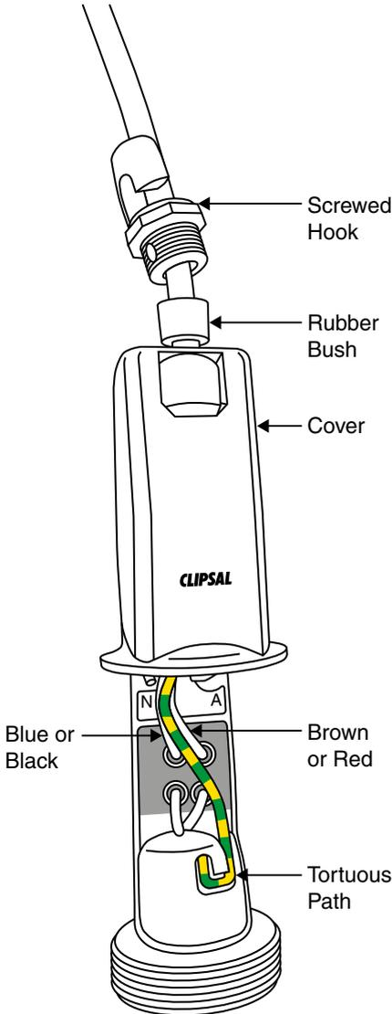
NOTE: Earth wire is connected directly to the socket and Active/Neutral are connected directly to the switch.
