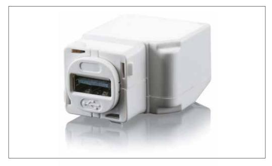
The Clipsal USB Charger Mech is designed to fit into 30 Series Aperture Wall Plates and Sockets, in both bracket and wall box environments. With up to 1.2A of charge current available, its smart-charging technologies ensure devices such as phones, tablets, cameras and eBook readers can be charged at the maximum safe rate governed by the device.
