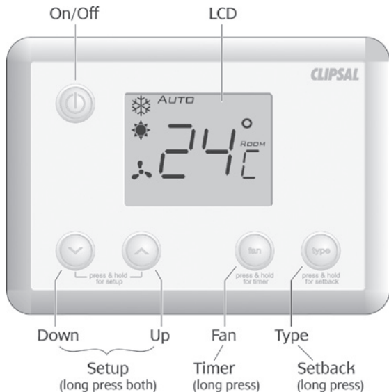
Figure 1. C-Bus® Single Zone Thermostat Front Panel
