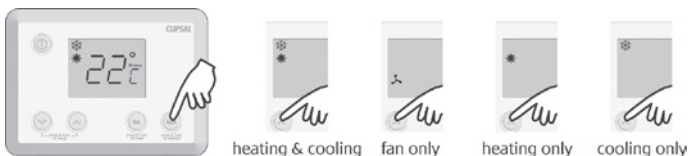
Figure 2. Operating Types for a Reverse Cycle or other heating and cooling system
