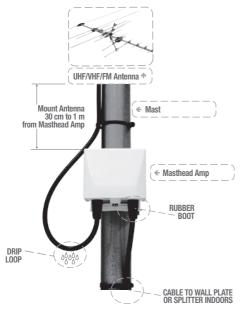
Masthead Amp Must be installed in this orientation to maintain weatherproof rating.
