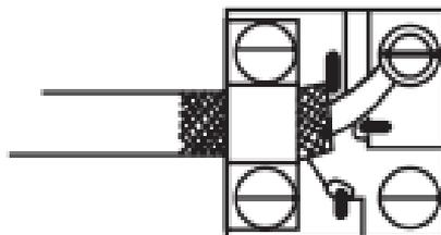
Pass cable under cable clamp and locate centre conductor in terminal hole, secure cable and conductor by clamping with screws.
