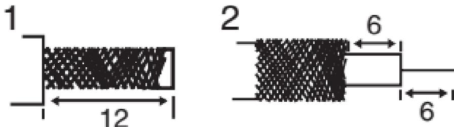
1. Strip off black outer casing 12mm from end of cable.
