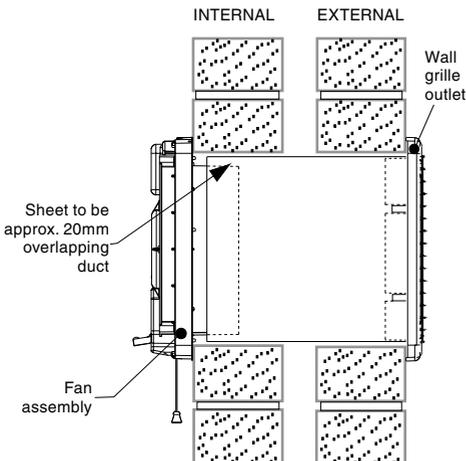
7. Place cover assembly as shown. Tighten retaining screw. Test. Ready to go.
