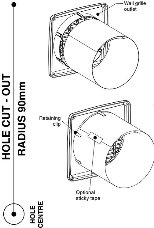
6. Screw wall grille outlet to external wall.
