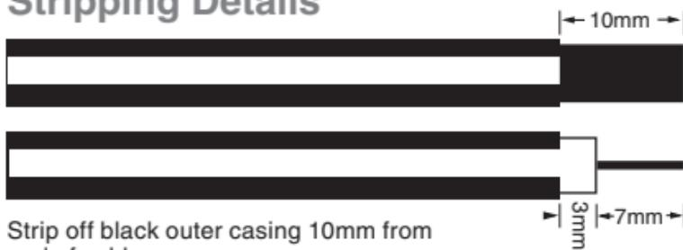
Strip off black outer casing 10mm from end of cable.
