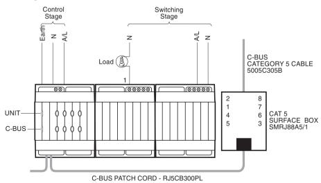
The DIN Rail Dimmer Unit is capable of handling up to eight channels of 1A dimmed loads. The installer should make adequate consideration for the total current consumption when selecting power feed cables. It is recommended that multiple feed cables to be allowed for.
