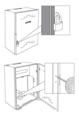
2. Drill holes at position indicated on frame.
