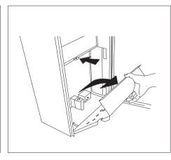
1. Locate bottom of security panel between inside front of box and bracket, then hinge into position.
