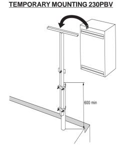
Lift enclosure onto bracket and fix into place. Tighten clamp securely.
