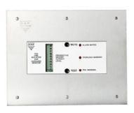
The Line Isolation and Overload Monitors (LIOM's) shall be the ESP Series catalogue no. E05 and shall comprise of an 18 segment Prospective Hazard Current (PHC) LCD Bargraph display, mutable two tone audible alarm activated at 5mA PHC and 15A/20A overload current, alarm muted – overload warning – PHC warning amber indicators, and in built test facility.
