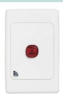
Each RCD shall have an Audible Alarm to highlight that the RCD has tripped. The Audible Alarms shall be the ML2000 Series catalogue no. ML2031E08 Series and shall comprise of a mutable two tone audible alarm, flashing red visual alarm, and mute push button labelled "press to mute"
