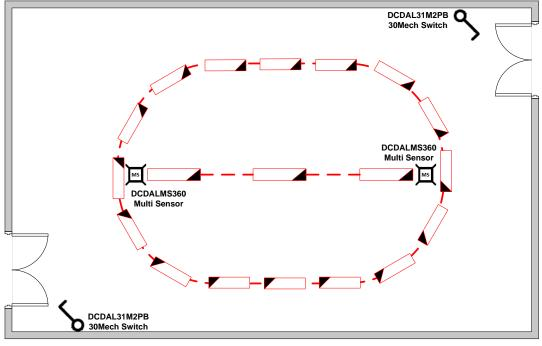
In this example, to meet the customers requirements, a DALIcontrol Native Solution is recommended. A DALIcontrol power supply is installed in a switchboard, which powers the DALI line. This two-core feed (DALI line) is connected to all your DALI devices, including switches, detector and lighting fittings.
