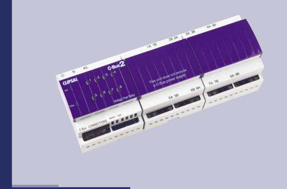
The L5508RVF Series units are C-Bus relayswitching devices designed to be mounted in electrical switchboards or similar enclosures. For ease of installation, they are DIN rail mounted, measuring 12 DIN modules wide. Eight independent voltage free relay contacts are provided for general switching applications.
