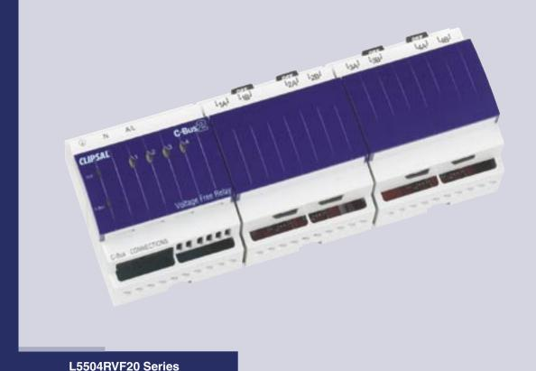
The L5504RVF20 Series Units are C-Bus relay-switching devices designed to be mounted in electrical switchboards or similar enclosures. For ease of installation, they are DIN rail mounted, measuring 12 DIN modules wide. Four independent voltage free relay contacts are provided for general switching applications.
