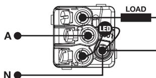
Two-way switching, no Neutral present LED 'ON' switch 'OFF'
