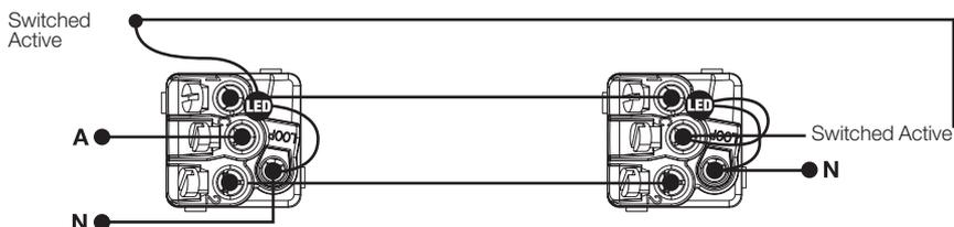
Two-way switching, Neutral present at the switch LED 'ON' switch 'OFF'
