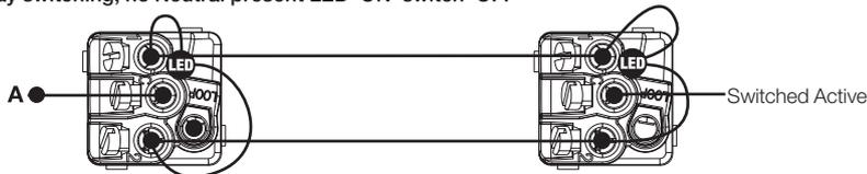
Two-way switching, Neutral present at the switch LED 'ON' switch 'ON'
