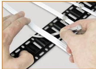
**2** Place cable in desired position. Thread cable tie through Cablemate™.
