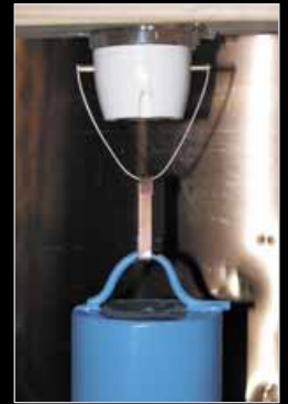
Supporting a 10kg (100N) load for 24 hours at 70°C
