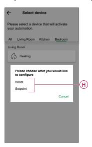
9. Tap **Setpoint**, set the required temperature using vertical sliding bar (I), then tap **Set**.
