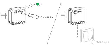
The shutter moves up and down for a few times. The status LED stops blinking green on the Wireless switch and the Puck. The Puck can now be controlled by the Wireless switch.
