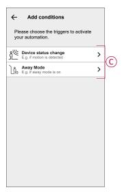
a. In this example, we will select **Device status change** and choose a device to set the condition. Then, we will select the state of the device that will trigger the automation, such as the closed state of a micromodule shutter.
