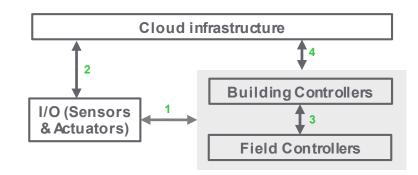
Each of these input and output data flows fall under one of three methods of communication via a wire using voltage/current/resistance signals, OT protocols, or IT and IoT protocols. Below we describe how sensors/actuators and controllers utilize these communication methods.
