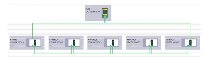
The ring topology can only be used with a media redundancy protocol (MRP) capable managed device.
