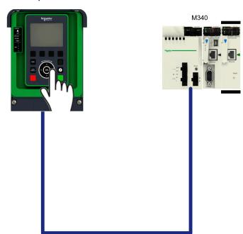
The drive is controlled from the communication but the frequence reference value is adjusted on the display terminal. The control word comes from the controller and is written according to CiA 402 profile.
