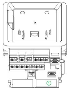
1 Fieldbus Module Slot A
