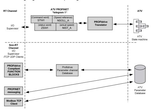
The following section describes how the system is operated when configured in PROFIdrive mode (telegram 1).
