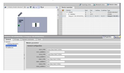
New parameters are added or modified by entering the drive Modbus address.
