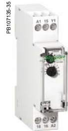
iRTC ■ Delays de-energizing of a load upon closing of an auxiliary contact (push button)
