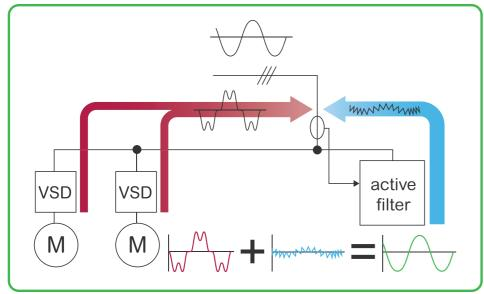
Figure 4: Simplified illustration of an active filter
