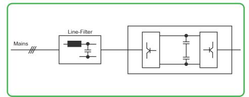
Figure 3: Simplified illustration of a low harmonic drive
