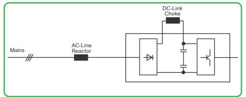
Figure 1: Simplified diagram of an inverter with AC line reactor and DC link choke
