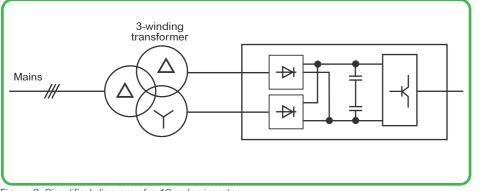
Figure 2: Simplified diagram of a 12-pulse inverter
