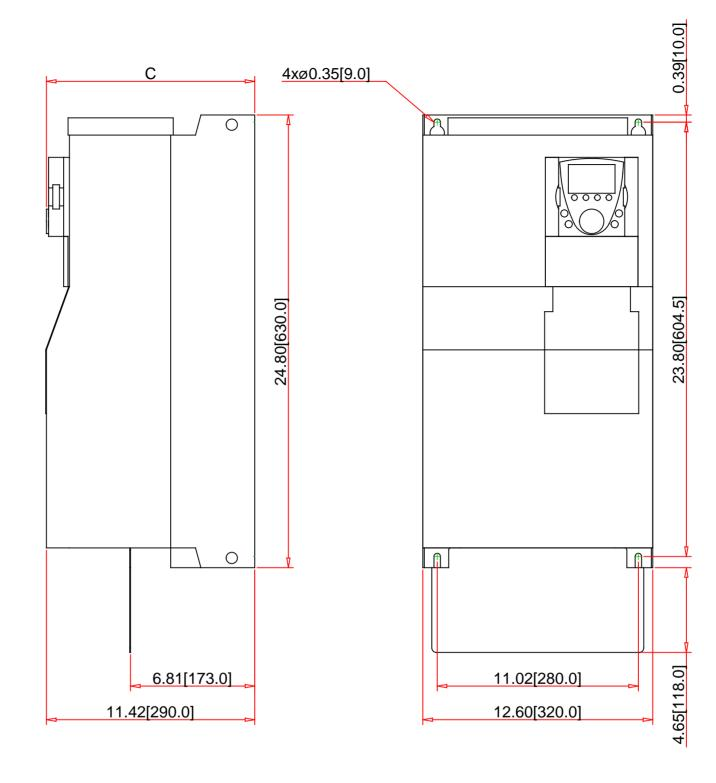
Optional EMC grounding plate is shown, it may be removed if not needed in the application.
