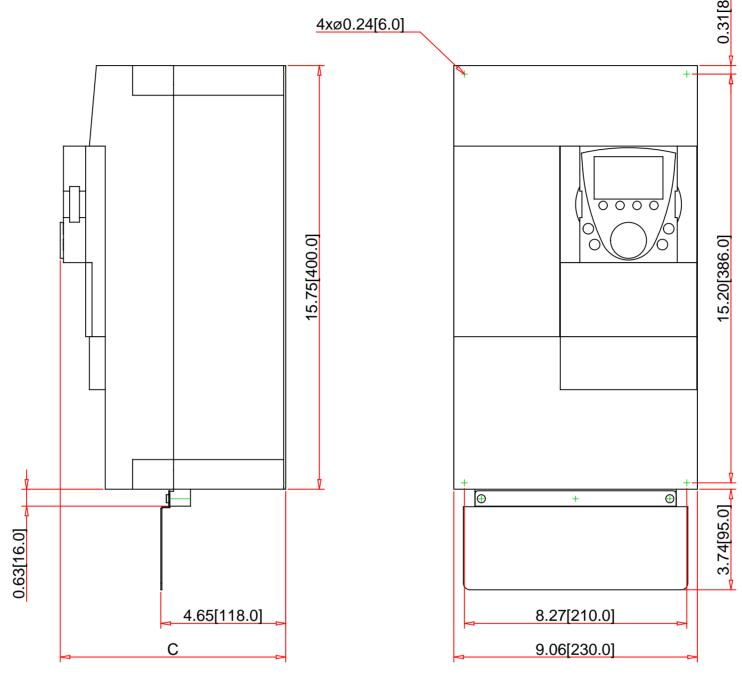
Optional EMC grounding plate is shown, it may be removed if not needed in the application.
