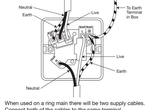
When used on a ring main there will be two supply cables. Connect both of the cables to the same terminal.
