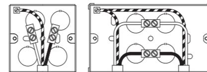
If the cable cannot be isolated, ensure that the bare ends of the live and neutral cables are terminated separately, within suitably sized terminal blocks. The terminal blocks should then be covered with insulating tape for additional safety. Any earth cables must be sheathed in green/yellow sleeving and connected to the earth terminal in the wall box. In all instances, it is important that the earthing circuit is maintained when removing an accessory.
