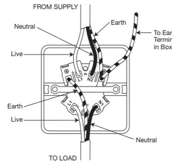
When used on a ring main there will be two supply cables. Connect both of the cables to the same terminal.
