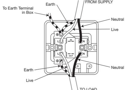
When used on a ring main there will be two supply cables. Connect both of the cables to the same terminal.
