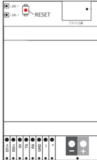
IP address after HW factory reset with HW button is always 192.168.0.10.
