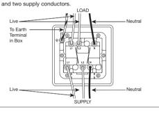
t the cables as shown in the wiring diagram.
