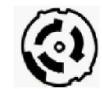
VIEW A CS8365C, 3P 4W, 50A(40A DERATED), 250V MAX, 3PH PLUG ENLARGED VIEW
