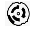
VIEW A CS8365C, 3P 4W, 50A(40A DERATED), 250V MAX, 3PH PLUG ENLARGED VIEW
