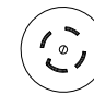
VIEW A NEMA L21-30P, 4P, 5W 30A(24A DERATED), 120/208V MAX, 3PH PLUG ENLARGED VIEW
