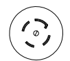
VIEW A NEMA L21-30P, 4P, 5W 30A(24A DERATED), 120/208V MAX, 3PH PLUG ENLARGED VIEW
