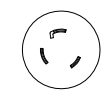
VIEW A NEMA L6-30P, 2P, 3W 30A(24A DERATED), 250V MAX, 1PH PLUG ENLARGED VIEW
