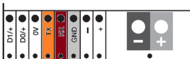
Picture 5 Wiser for KNX terminals connection
