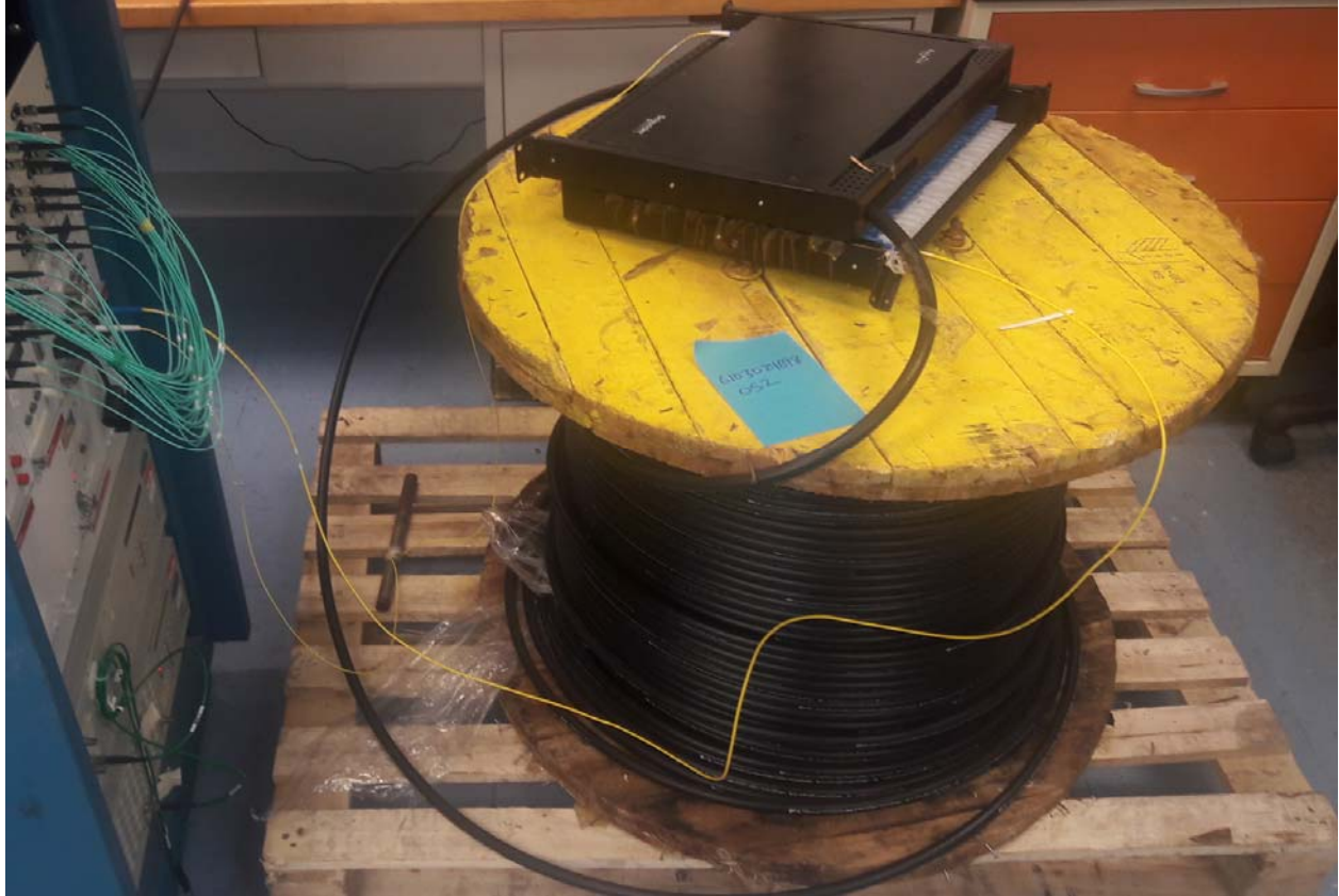
Figure 3: LC-SC OS2 Fiber Channel Test Setup
