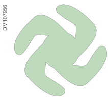
Specific Contacts Shapes Inside Vacuum Interrupters
