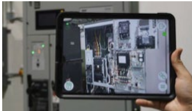
Figure 21. XR enables a technician to see behind the door of an electrical cabinet with “x-ray vision” for increased safety
