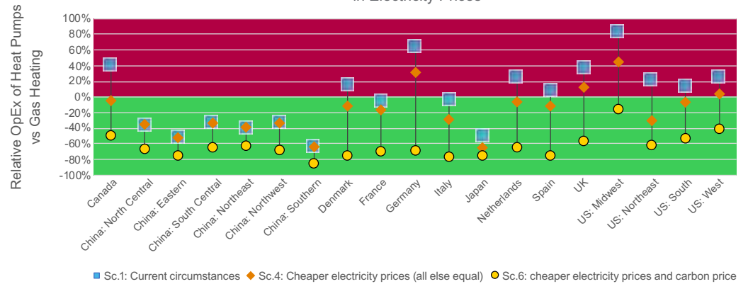
Figure 8: Heat Pumps vs Gas in Commercial New Builds Following a Change in Electricity Prices
