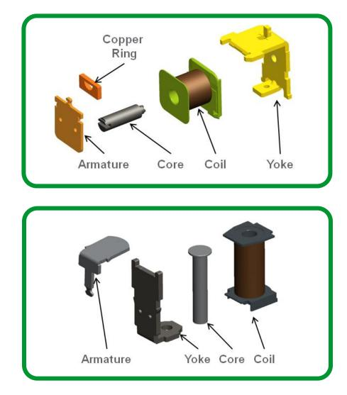
Figure 4a RXM Electromagnetic System
