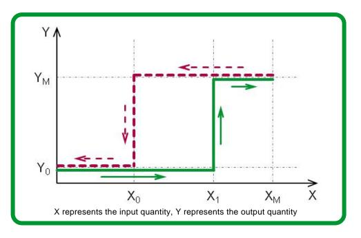
When the input quantity X starts to decrease along the dashed arrow direction from XM, the output quantity Y keeps the constant value Y=YM. But when the input quantity X decreases to X=X0, the output quantity Y jumps from YM to Y0.
