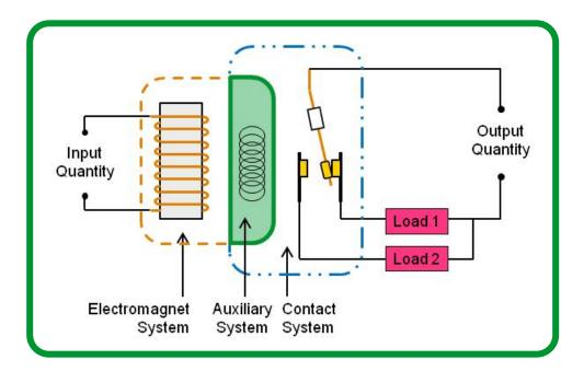
In **Figure 1**, the electromagnetic system is the sub-system inside the relay that receives the input quantity of current and voltage. When a voltage is supplied to it, the electrical current going through the coil generates the magnetic flow in the electromagnet system. The magnetic force, which is produced by magnetic field, stimulates the auxiliary system to drive the contact system.
