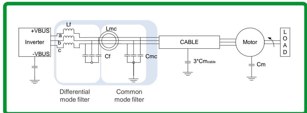
If the Sinus filter is associated with a common mode filter, this allows for the suppression of bearing currents (see **Figure 6**) and the reduction of the conducted EMC disturbances to the mains. The combination of those two filters presents the most robust solution for avoiding VSD-to-motor connection issues. This solution is also very cost effective if a long motor cable is used as long as a shielded cable is not required.
