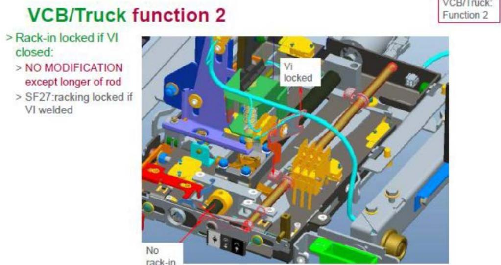
The racking truck guide rails are the only interface elements necessary to guarantee the reliability of the Circuit breaker plug-in function on the plug-in bushings of the MV cubicle.
