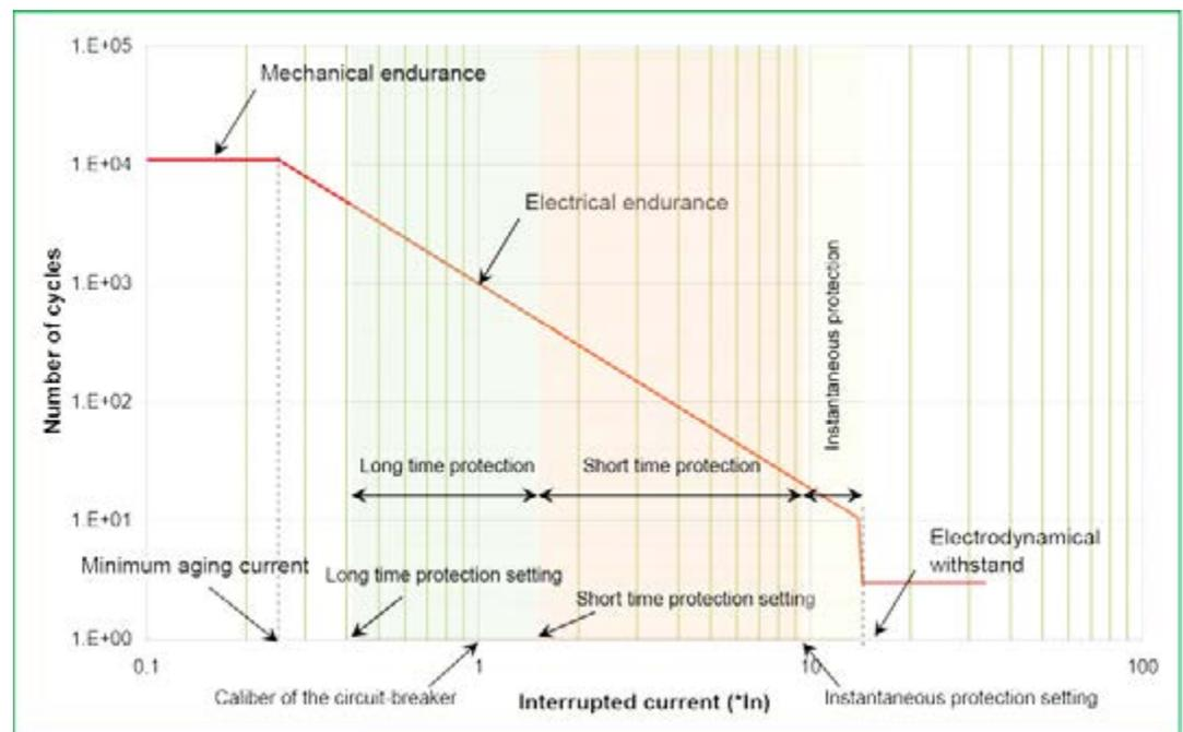
The data indicates that high interrupt currents significantly reduce the lifespan of the breaker (specified the number of cycles of operation). Also, circuit breaker aging is not impacted by current if the interrupted current is below the minimum aging current specified for the device. Under this condition, lifespan is based solely on the mechanical endurance of the device.
