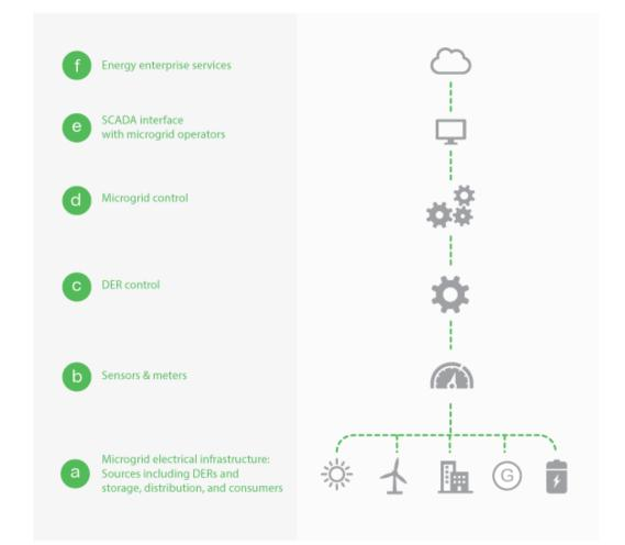
Microgrid functional architecture, from the grid to the cloud
