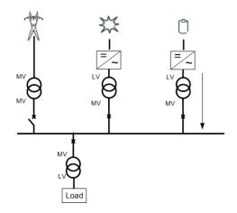
As microgrid operating conditions change, the network topology also changes. Consequently, the short-circuit current capacity may vary both in magnitude and direction. Protection systems have to be carefully designed in a way to secure people and equipment from all possible types of fault in each operating mode, while avoiding downtime due to errant protection discrimination.
