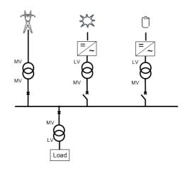
B. Supplied by the grid and a local energy source in parallel, storage is recharged
