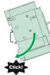
TeSys GV4 can be mounted on a backplate or on a DIN rail (35 or 75 mm).
