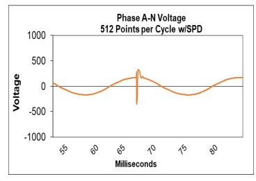
The waveforms in **Figures 7 and 8** illustrate the SPD did attenuate the transient event's peak voltage. However, once again the sampling rate does not necessarily allow reliable conclusions to be made regarding the actual magnitude of attenuation.
