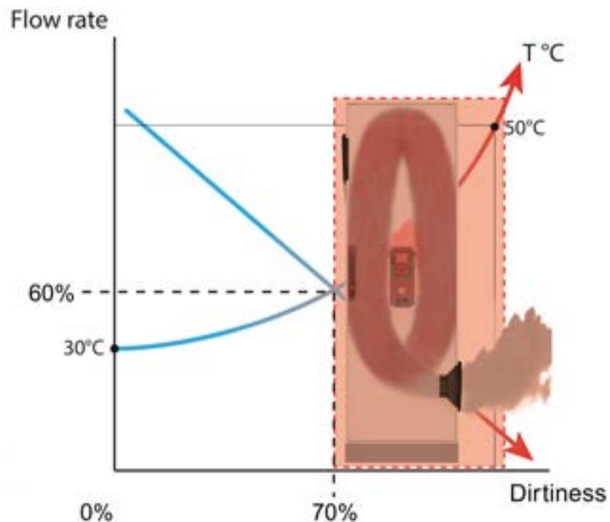
Equipment health is directly dependent on filter dust levels. Clogged filters cause fans to run inefficiently, airflow to slow or stop, and equipment lifespan to be cut in half.
