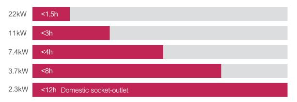
Based on average charging duration for Renault Zoe with 24 kWh battery
