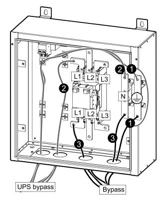
4. Disconnect the signal cable E31 from the L2 busbar of the power contactor. Reconnect the E31 signal cable to the neutral busbar.
